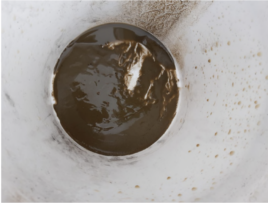
Plate 1: View of silt recovered during attempted purge of BH514A on 3 rd February 2022
