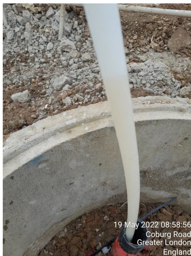
Plate 3: Views of groundwater within a VOC vial and Waterra tubing collected during the sampling round of 19 th May 2022. The level of silt has become much reduced in recent sampling rounds
