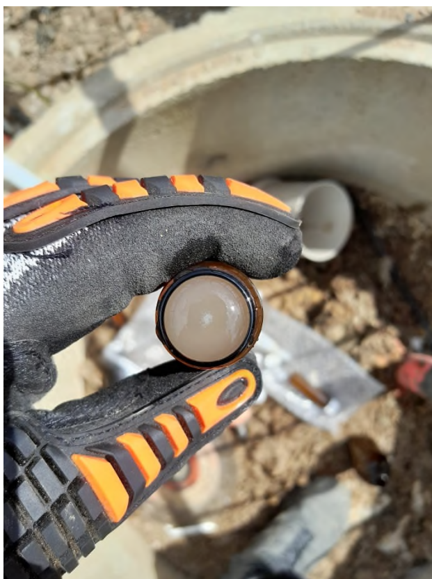
Plate 3: Views of groundwater within a VOC vial and Waterra tubing collected during the sampling round of 19 th May 2022. The level of silt has become much reduced in recent sampling rounds
