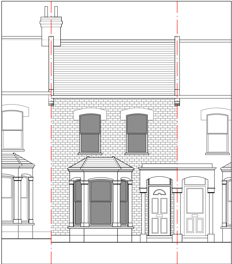
EXISTING FRONT ELEVATION (WEST) SCALE 1:100 @ A3
