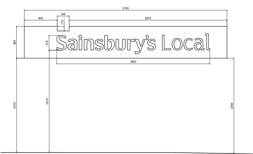
01 PROPOSED FASCIA SIGNAGE-INTERNALLY ILLUMINATED- ILLUMINATION LEVEL - 375 cd/m 2 P 94621 213 1:50@A3
