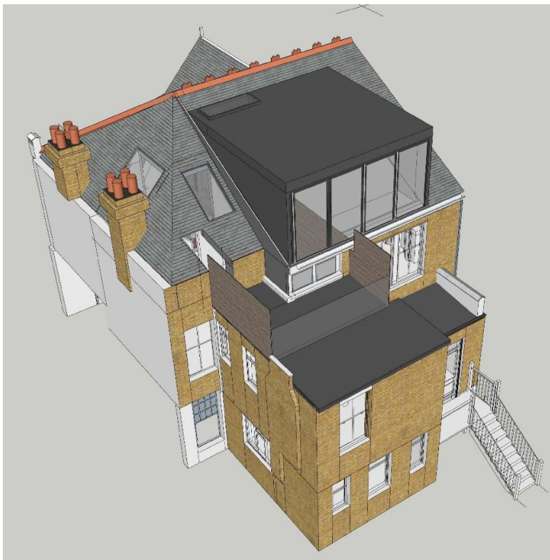
Rear view of proposed rear roof extension
