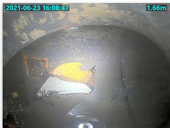
Fig 3.1: Line 6, hole in pipework
