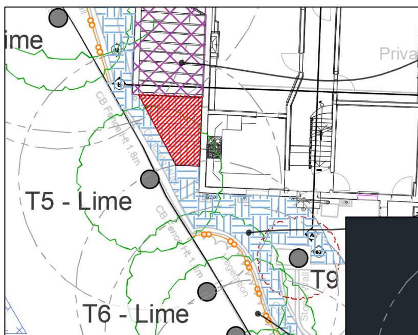
Figure 3 (left): Largest area of proposed relative impact within a standard circular RPA where proposed development sees an increase of intensity and change of context from hard surfacing to building foundation
