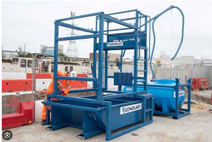
Figure 6 Concrete wash out
