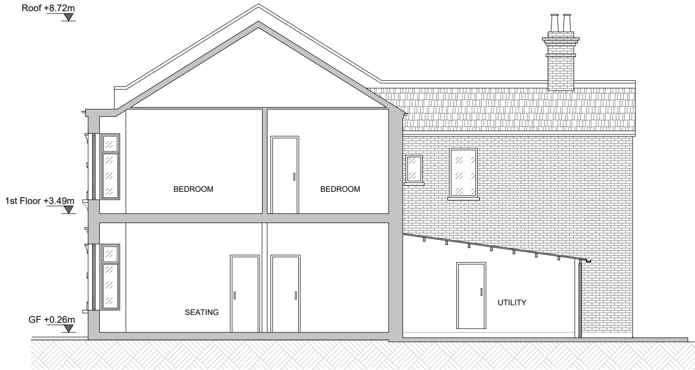
EXISTING SECTION - A -A scale 1:100
