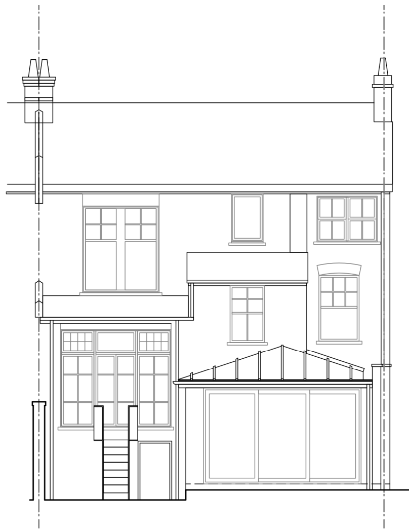
02 Existing South (Rear) Elevation
