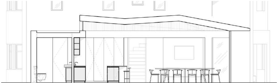
Section AA (extract) from application for Pre-Application Advice (PRE/2023/0025), indicating a folded-form roof.
