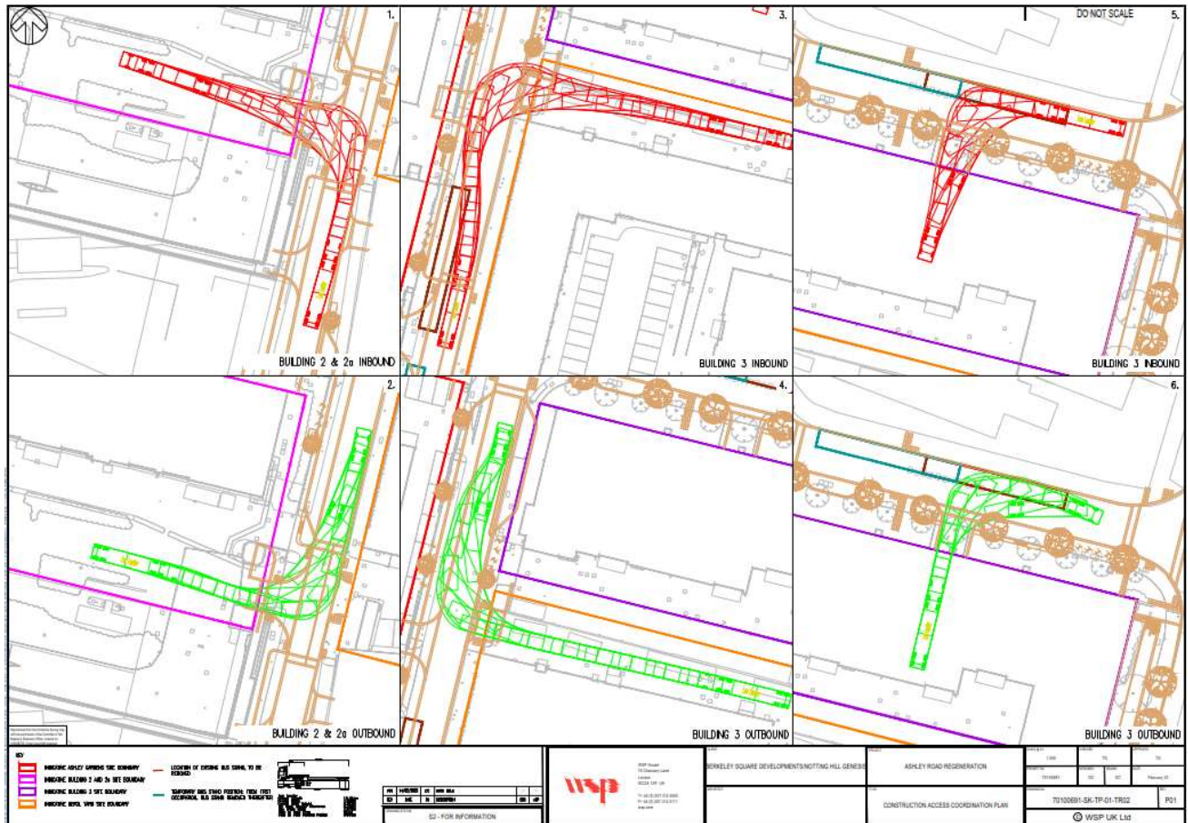
Figure 4-6 – Low Loader accessing the site
