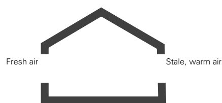
Typical building section demonstrating passive cross ventilation.
