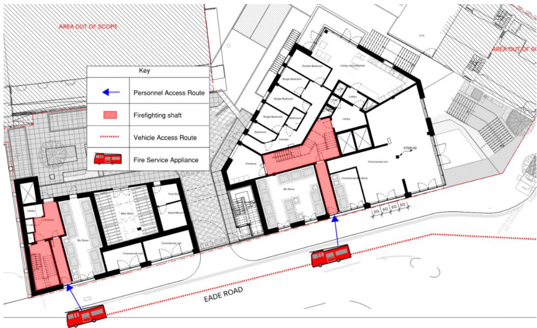
Figure 3.3 Fire Service access to ground level
