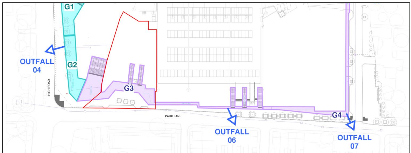
Figure 3-3: Surface water catchments ground level 00
