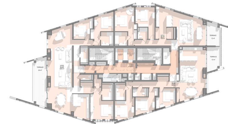
FIGURE 252. Typical Residential Floor - Level 19-25 (Accessible)
