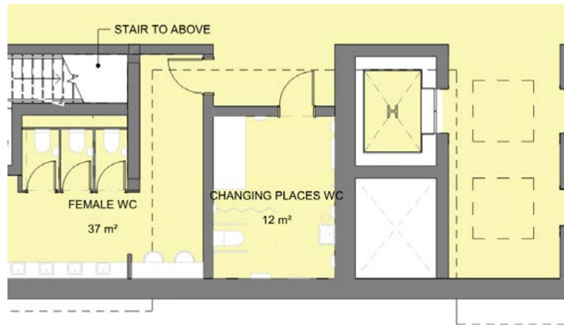
Figure 2—11 Changing places toilet facility
