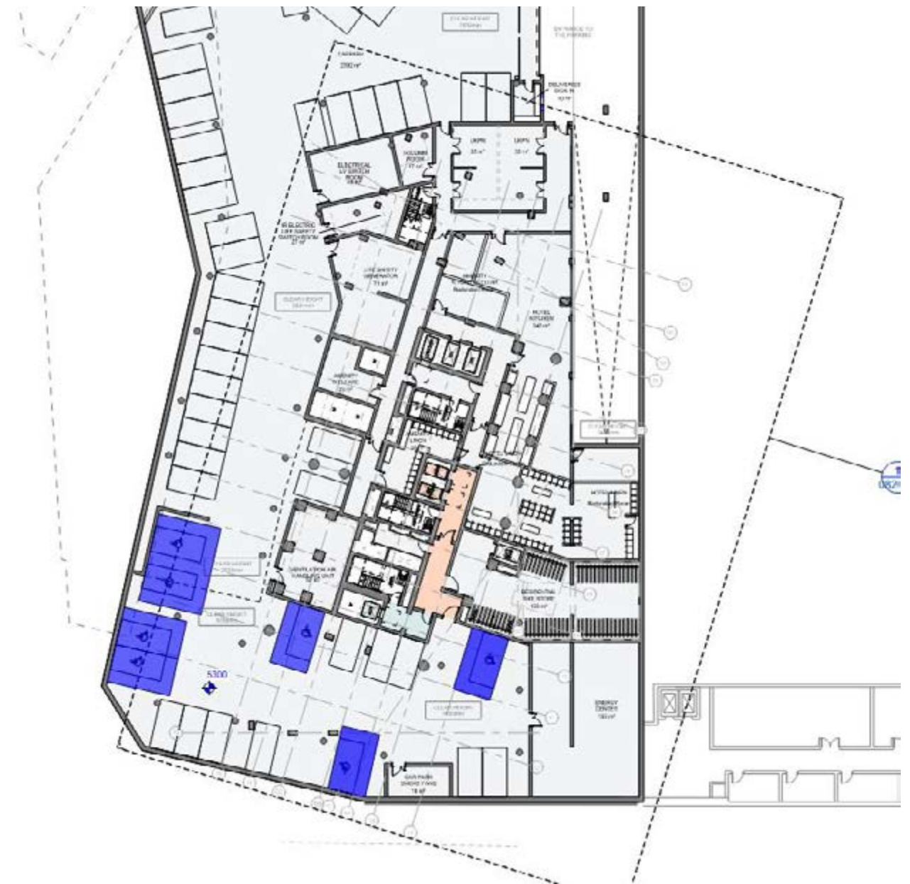
Figure 2—2 Accessible car parking spaces locations (Blue)
