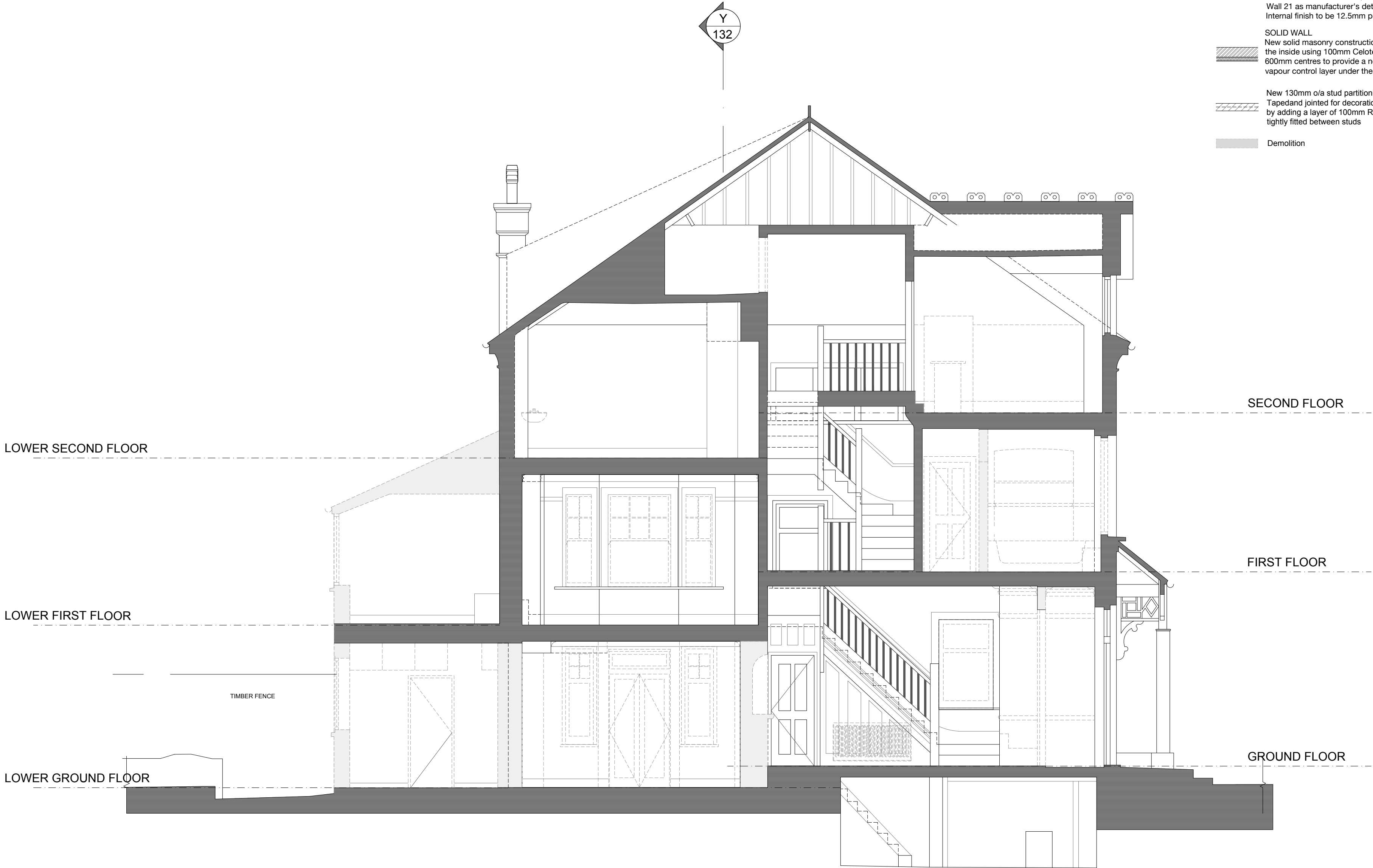
EXISTING & DEMOLITION SECTION X-X
