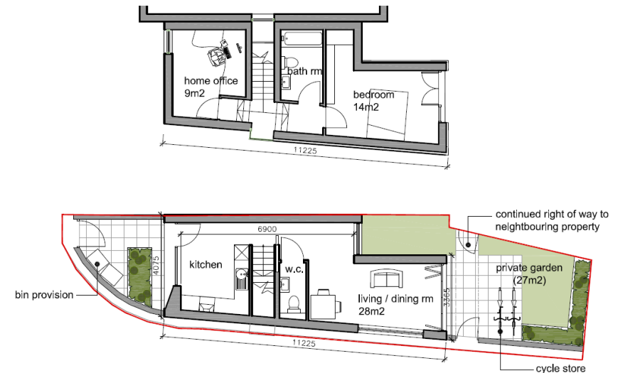
Fig11: ground and first floor plans
