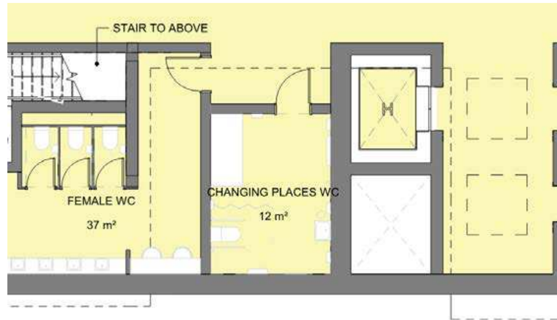
Figure 2—11 Changing places toilet facility
