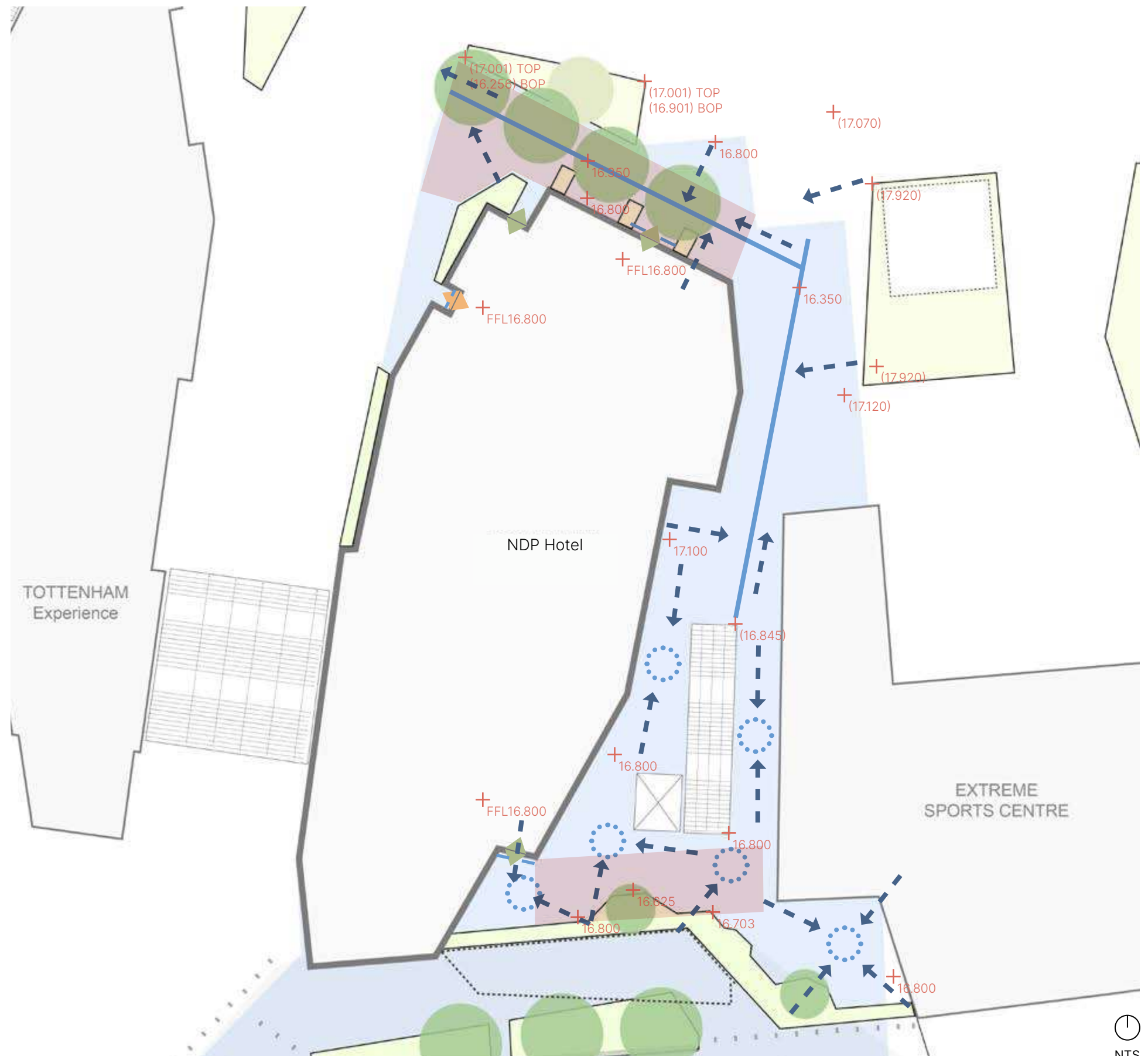
FIGURE 279. Drainage strategy for the Podium L01
