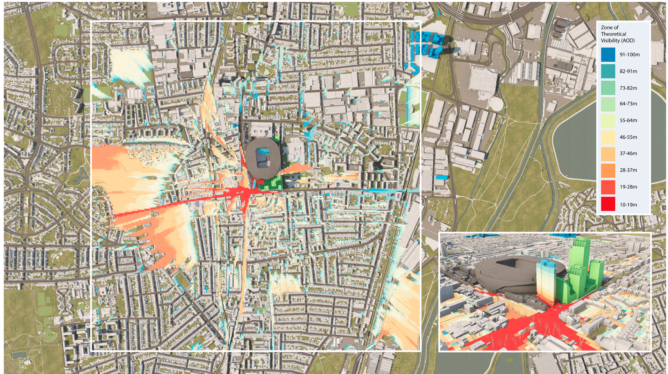
Fig.A3.1: ZTV diagram illustrating the theoretical visibility of the approved hotel (Plot 3) within the masterplan, covering an area of up to 2km in distance. The ZTV diagram reflects different height bands, with each colour identifying how much of the approved hotel building can be seen from any given location. The constructed elements of the Consented Scheme, i.e., Plots 1 and 2, are shown in grey. The approved schemes at Plots 4, 5 and 6 are shown in green. The ZTV diagram does not take into account trees as described in paragraph 2.69(iv) in section 2.
