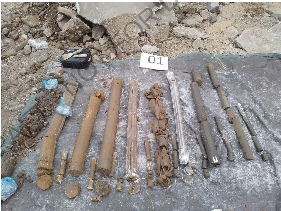
Soils encountered at BH01
