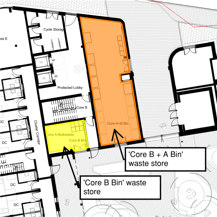
Figure 8 ‘Core B + A Bin’ waste store and ‘Core B Bin’ waste store locations
