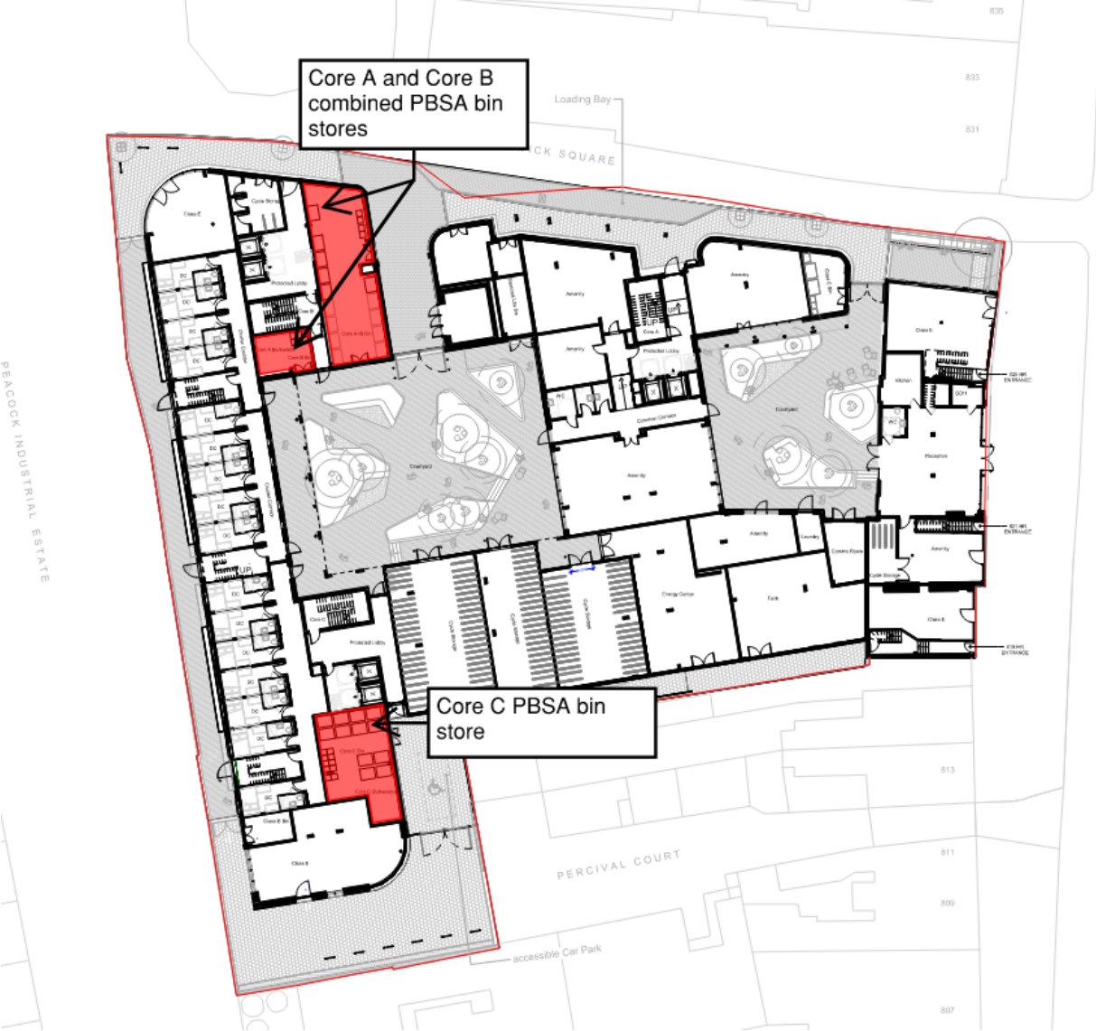
Figure 11 PBSA waste store locations
