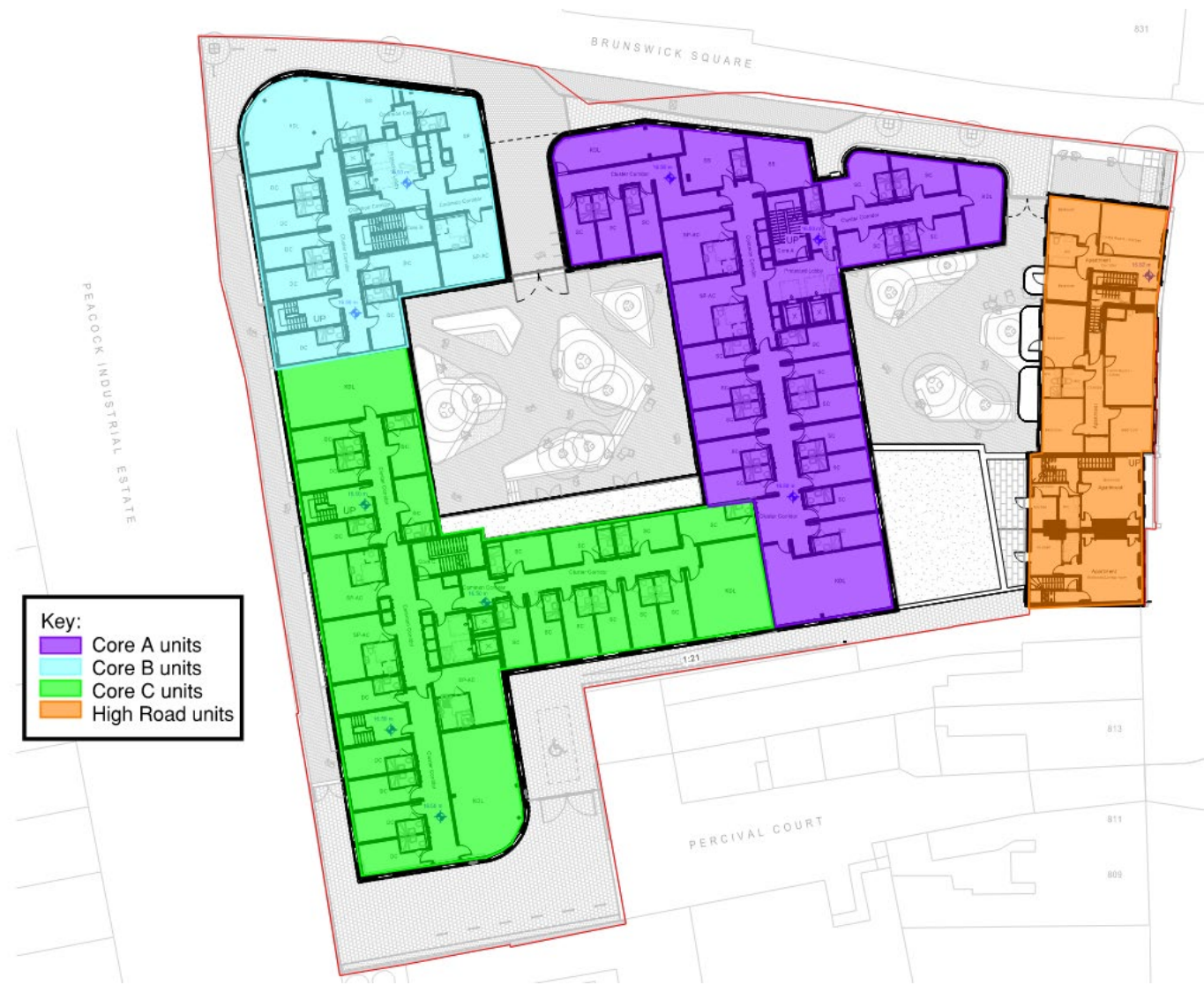
Figure 2 PBSA units (typical arrangement at Level 01)
