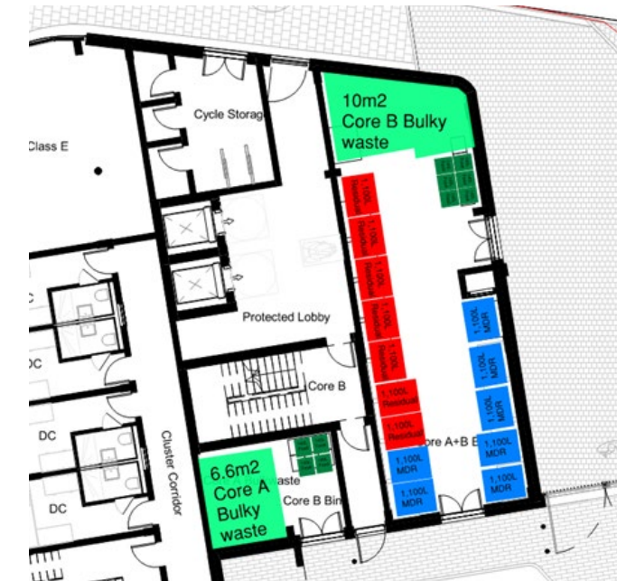
FIGURE 318. Core A/B PBSA waste store layout
