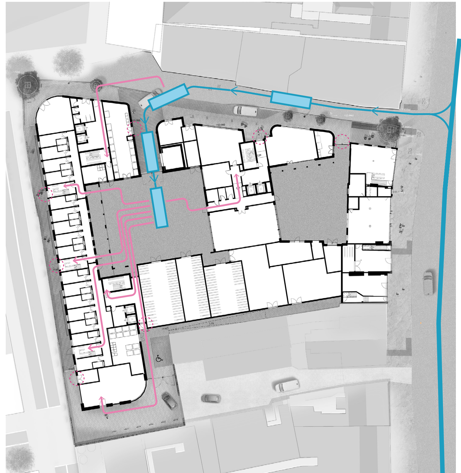
FIGURE 309. Ground Floor Fire Strategy Diagram
