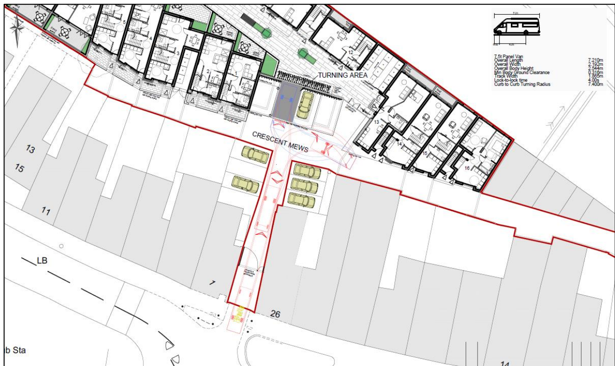
Fig 8: Site Access Post Superstructure Works
