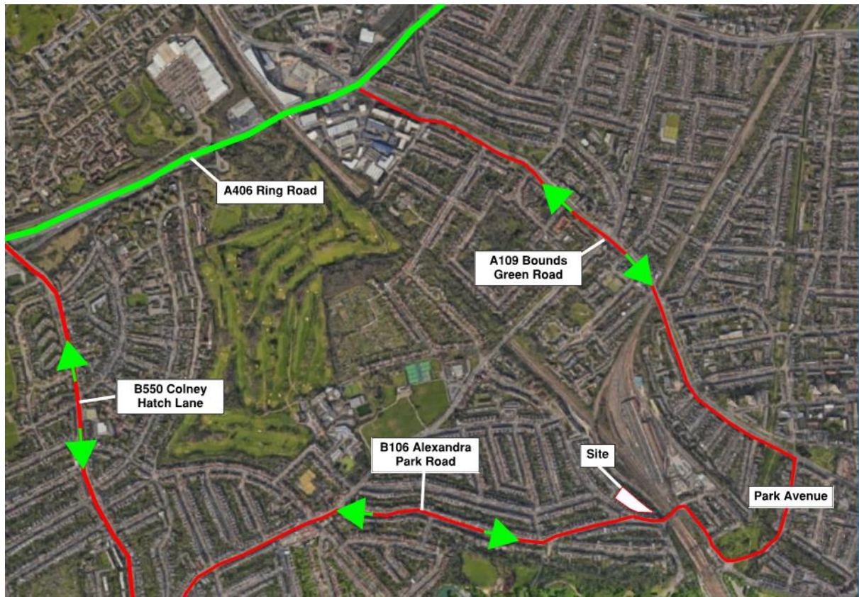
Fig 9: Proposed Construction Vehicle Access Route
