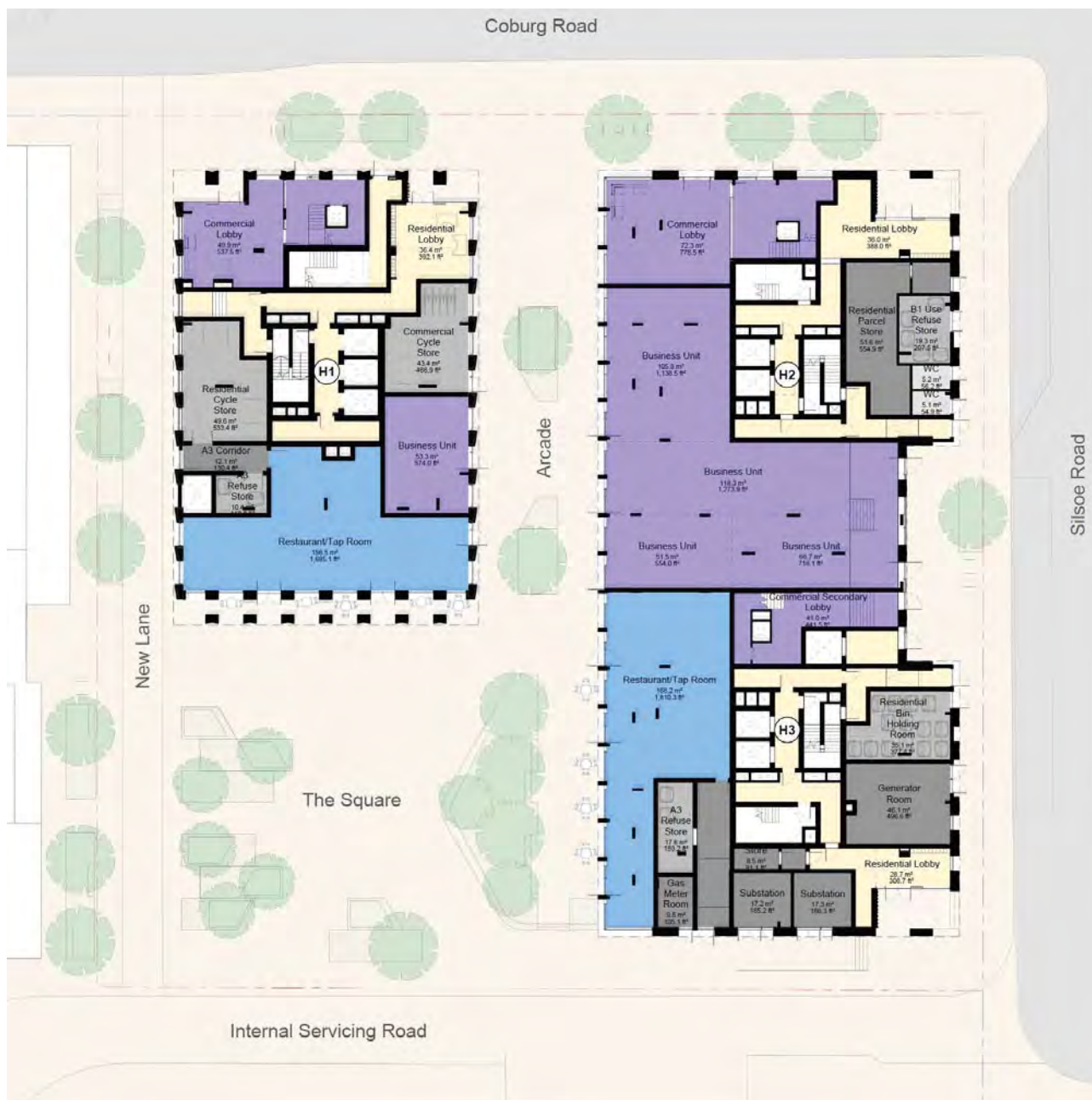
Figure 3.1: Ground floor layout of Block H1-H3 (Drawing No. 6726-SRA-ZZ-00-DR-A-SK102)
