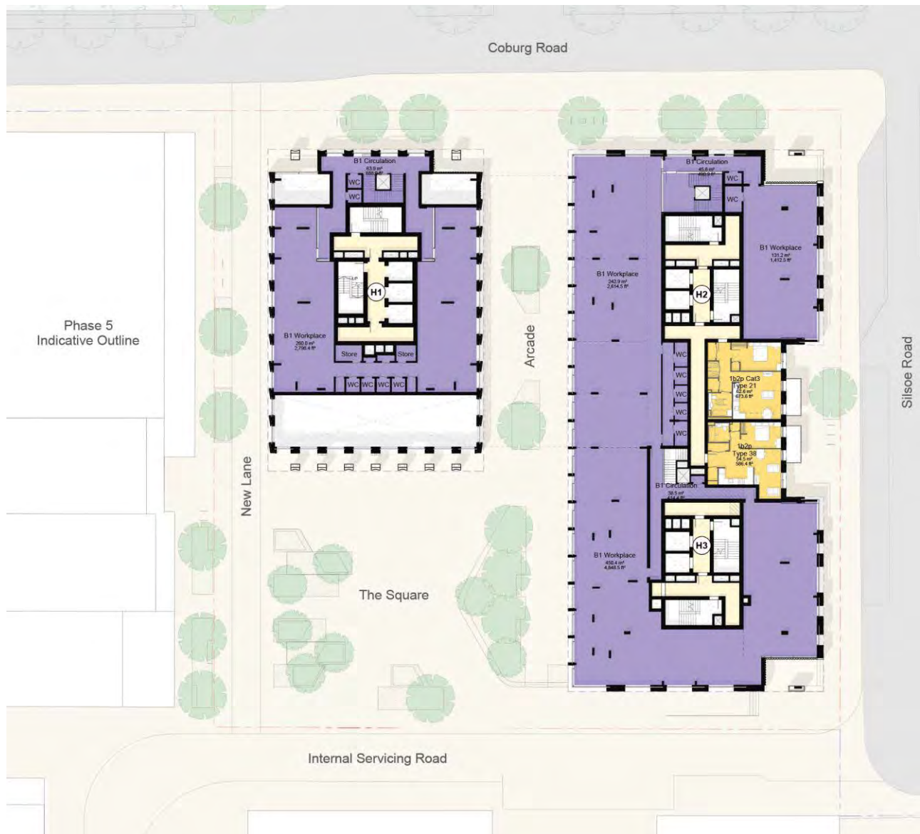
Figure 3.2: First floor layout of Block H1-H3 (Drawing No. 6726-SRA-ZZ-01-DR-A-SK103)
