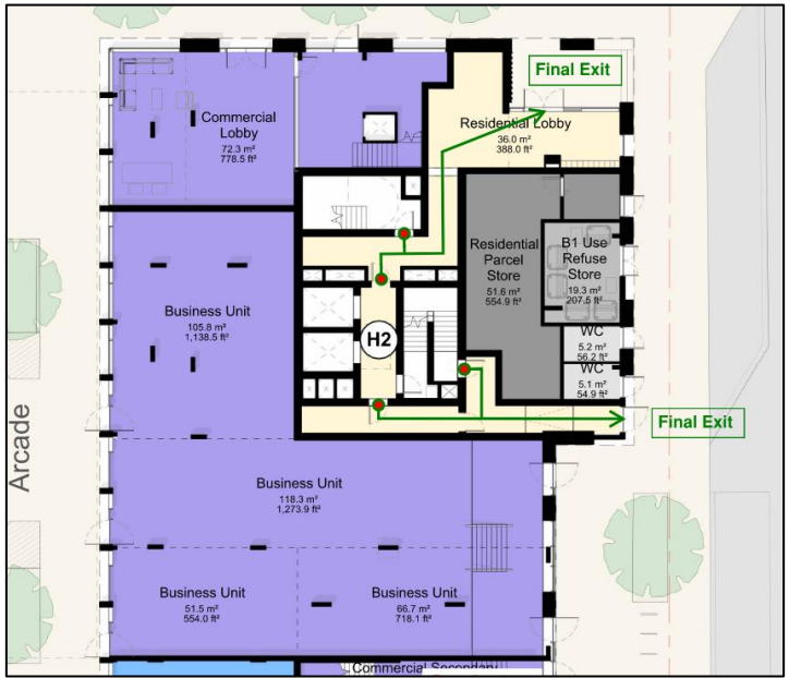
Figure 7 - Final exit route – Blocks H2
