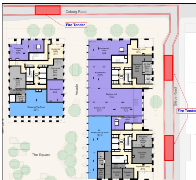
Figure 14 - Fire Tender Access Routes
