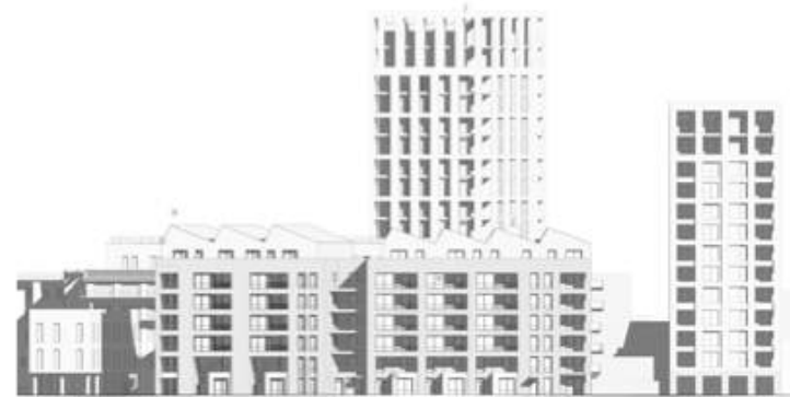
Example elevations of Block E (West) showing the proportion of glazing on the façade.
