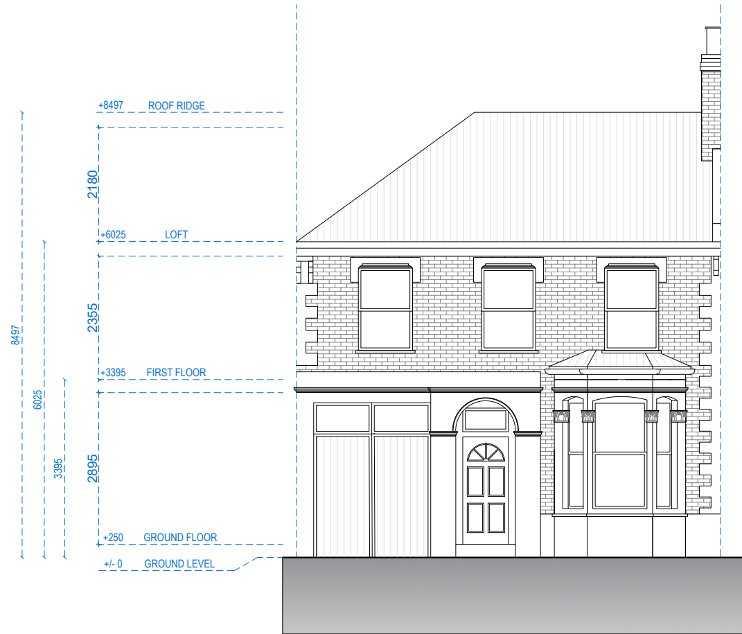
FRONT ELEVATION NORTH ELEVATION
