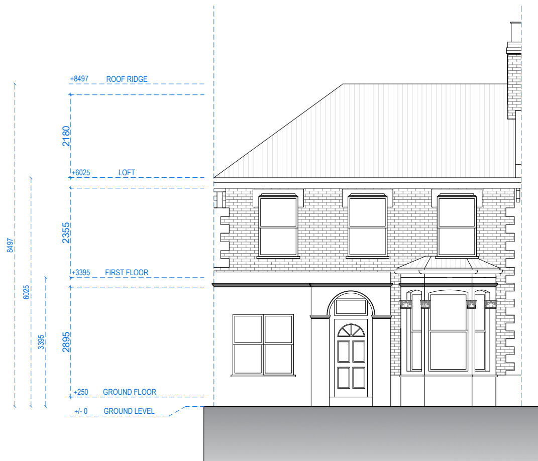
FRONT ELEVATION NORTH ELEVATION
