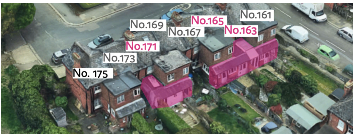
Image from the Office S&M DAS showing, in magenta, the later ground floor alterations. The first floors of the outriggers have also been extended and have flat roofs. These are not historic.
