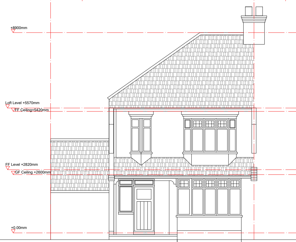
EXISTING FRONT ELEVATION
