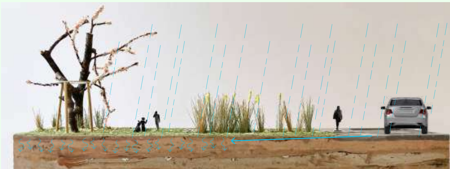
Elevation model of the Wood Green Common system, showing how the channel carries rain from the road to irrigate green spaces.
