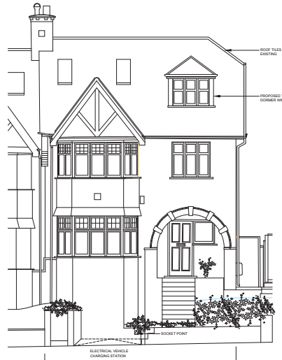
After - Extensive development at roof level, visible from front
