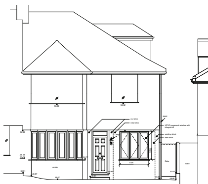
After - Garage door replaced with window
