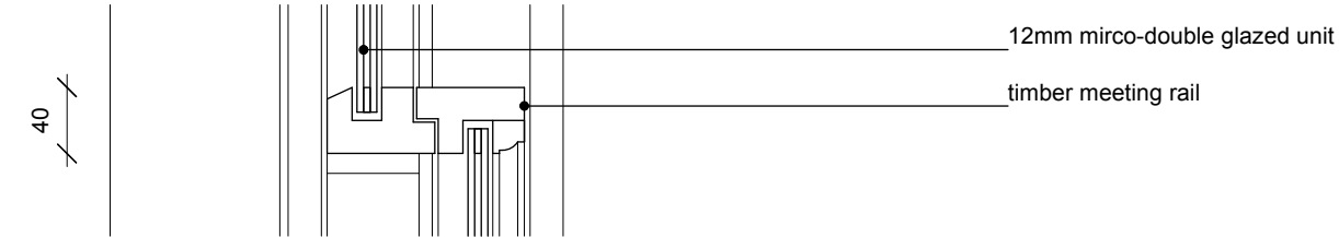
SASH WINDOW TYPICAL MEETING RAIL SECTION DETAIL
