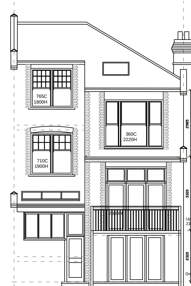
EXISTING REAR ELEVATION
