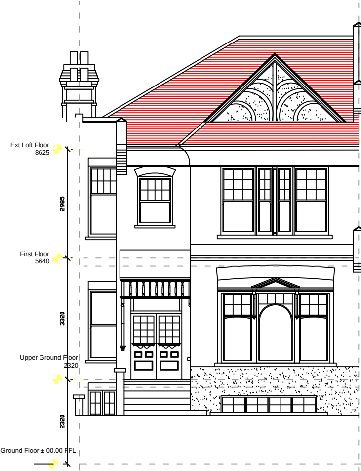
EXISTING FRONT ELEVATION
