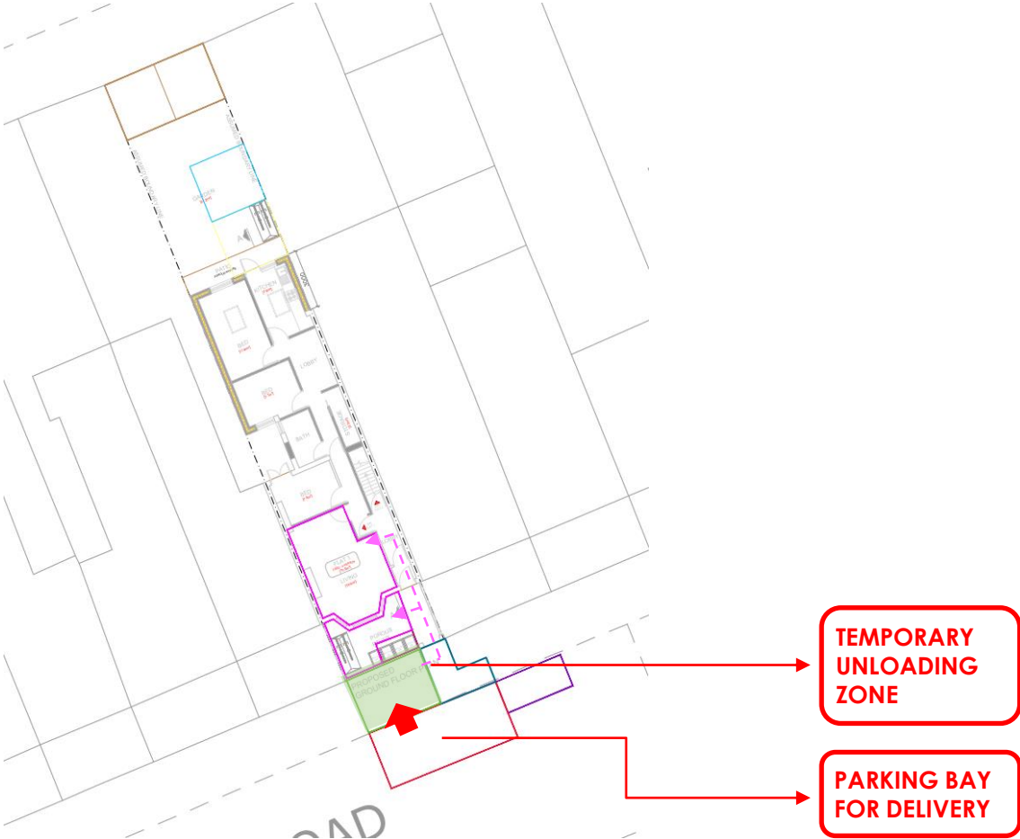
FIGURE 04 – LOADING AND UNLOADING MATERIALS ZONE
