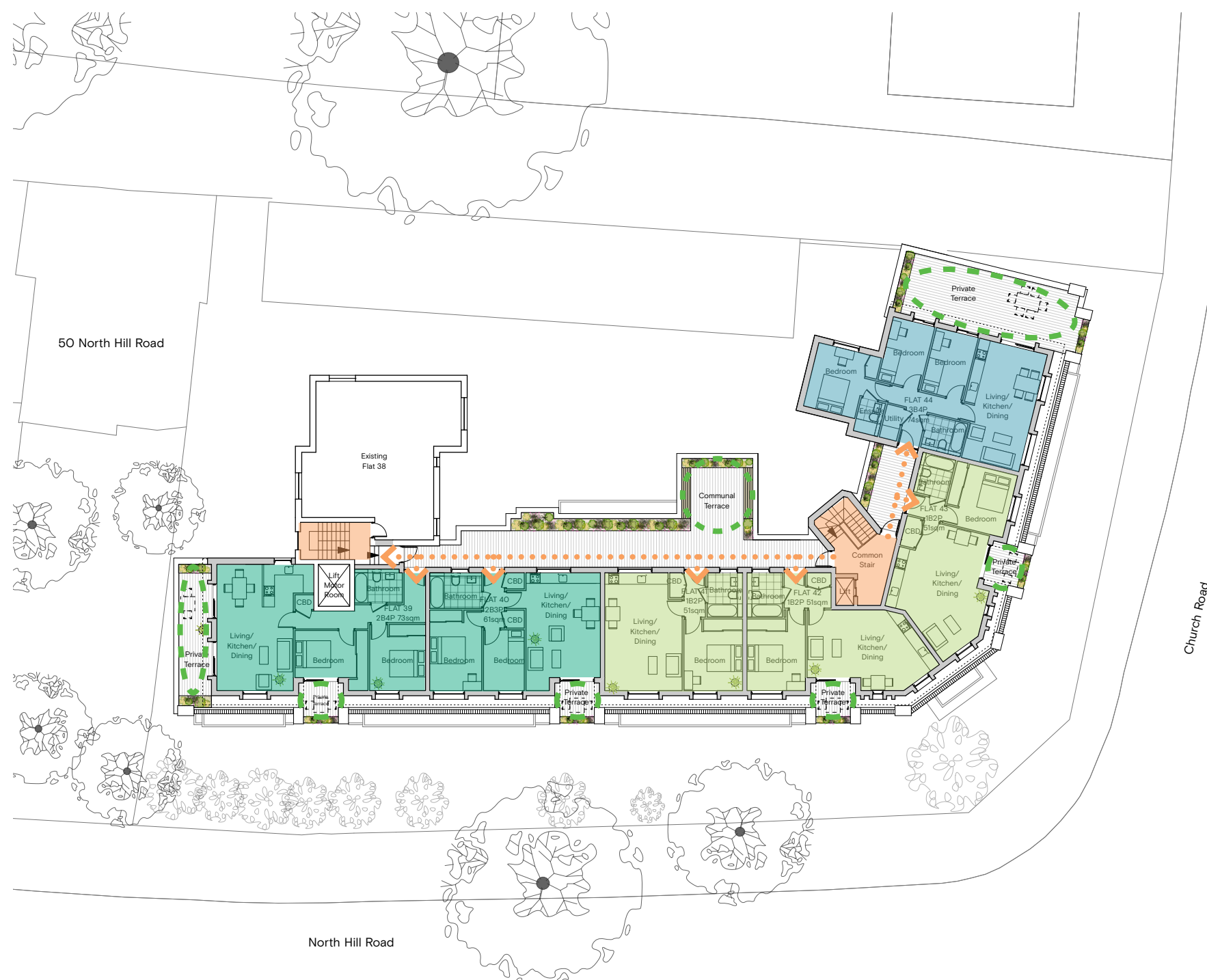
Figure 31: Proposed 4th Floor Plan showing the proposed access, types of accommodation and position of the amenity space
