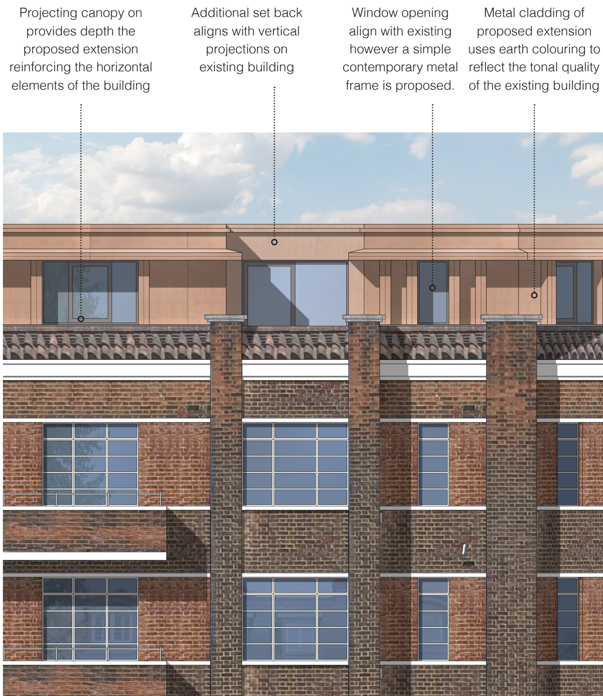
Figure 29: Front elevations bay study showing the materiality of the proposed extension in the context of the existing
