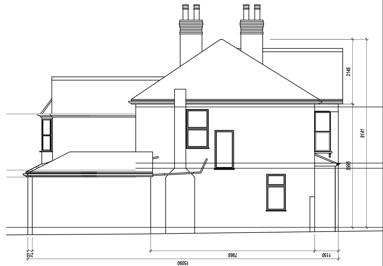
EXISTING Side Elevation (North West)
