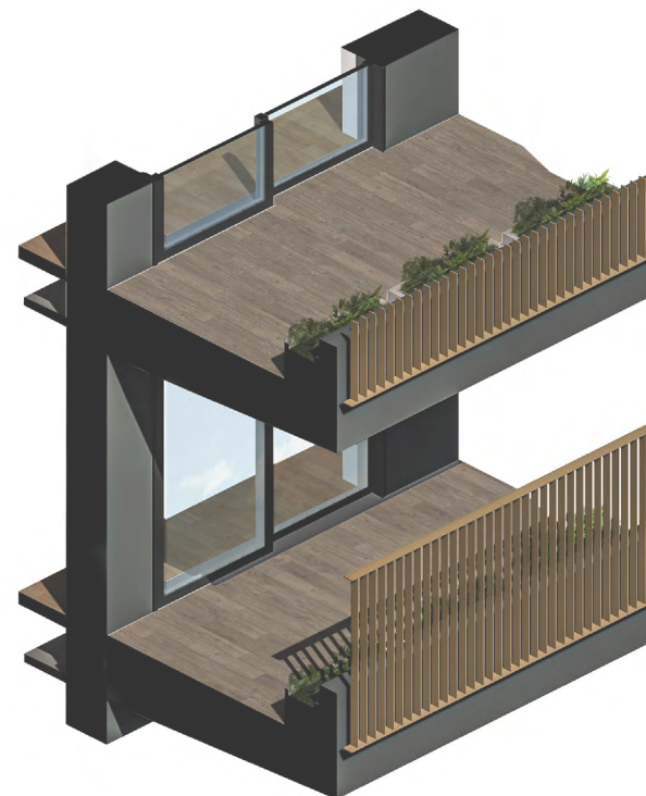
FIGURE 35. Proposed Scheme Revision - Wall Type 04 Recessed Infill Balconies Axonometric
