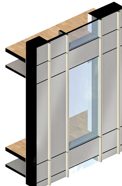
FIGURE 43. Proposed Scheme Revision - Wall Type 01 Planar Blade Axonometric
