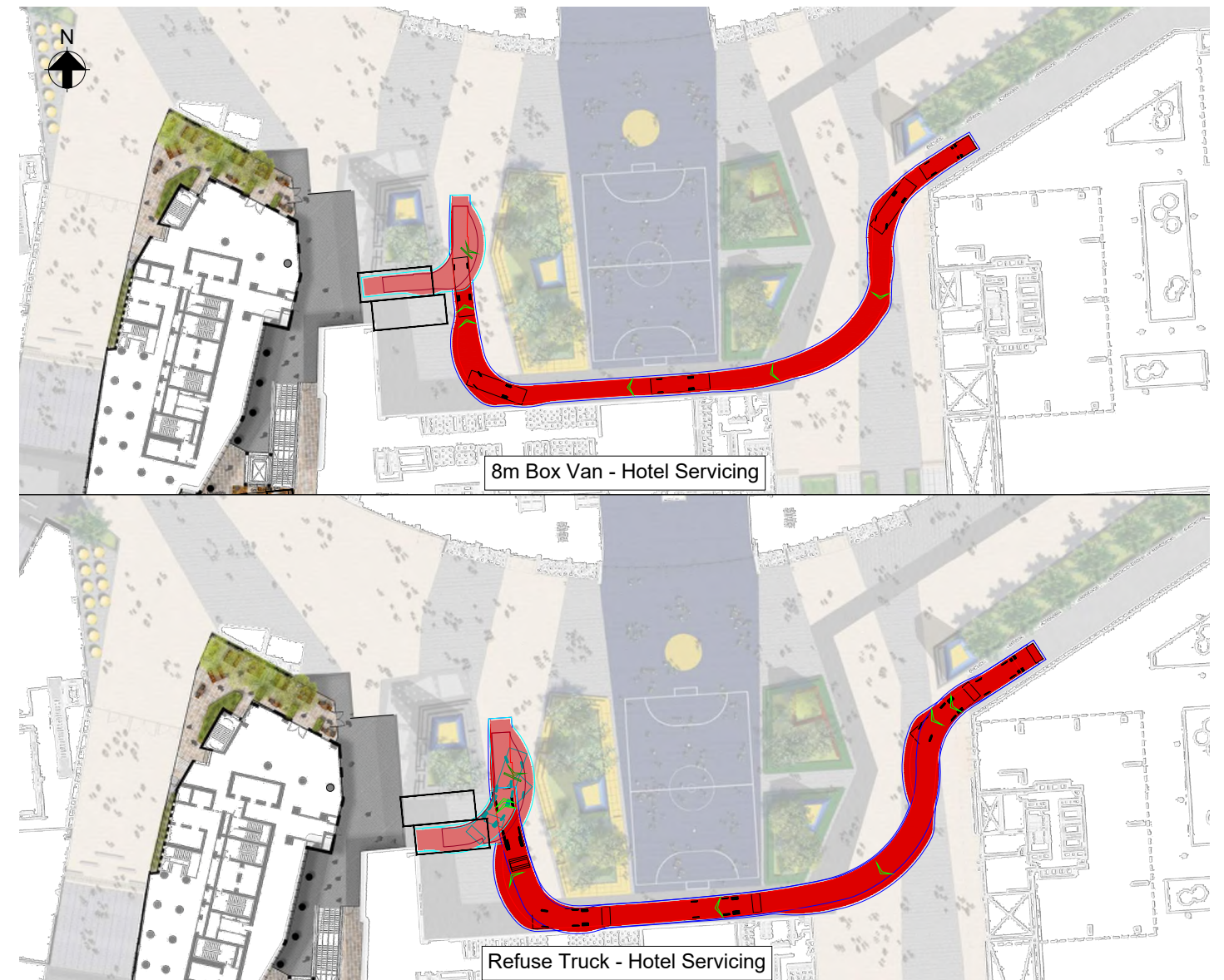
FIGURE 127. Delivery and Servicing - Podium Level Vehicle Tracking
