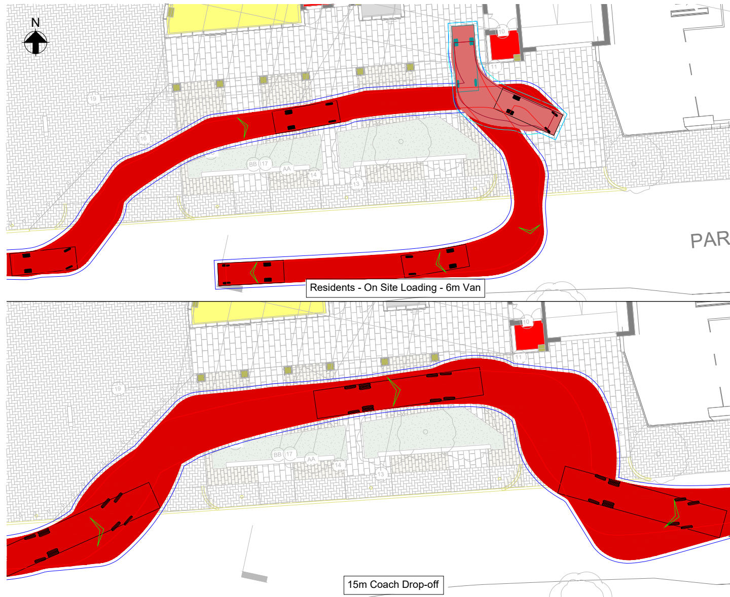
FIGURE 126. Delivery and Servicing - Ground Floor Vehicle Tracking
