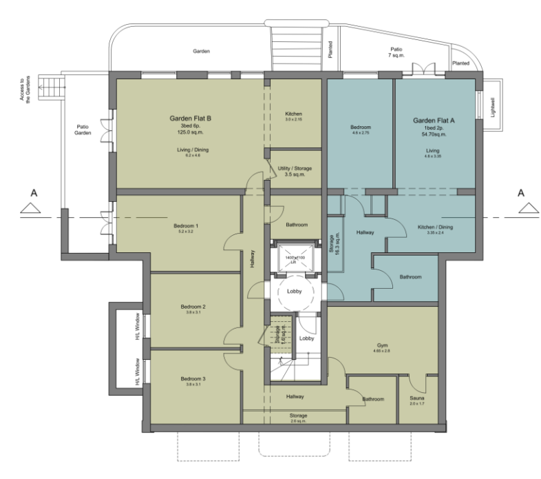
Figure 3: Proposed Basement Layout under Building Footprint (extract from Architect's drawing)
