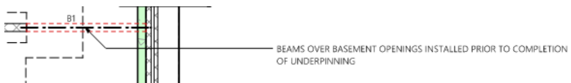
Figure 4 – Steel Beam Supporting Existing Masonry Wall
