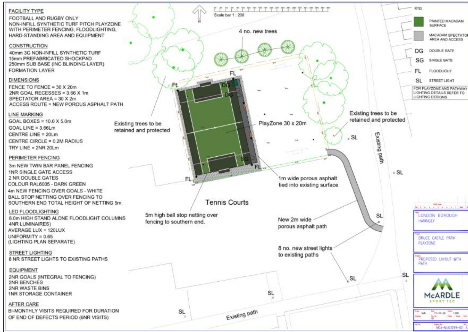
Figure 3: MCA-MUK3299-01 rev E – Proposed Layout. McArdle Sport Tec Ltd.
