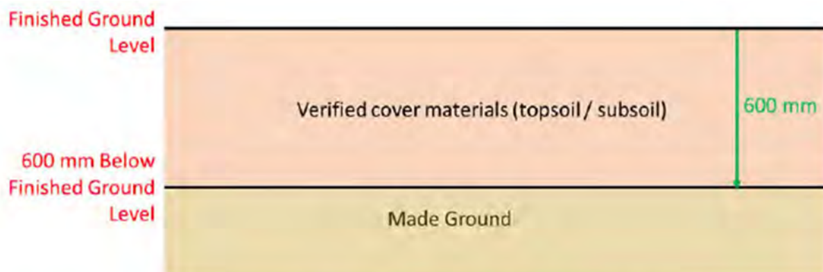
Clean cover layer conceptual cross-section (in areas of private residential garden)
