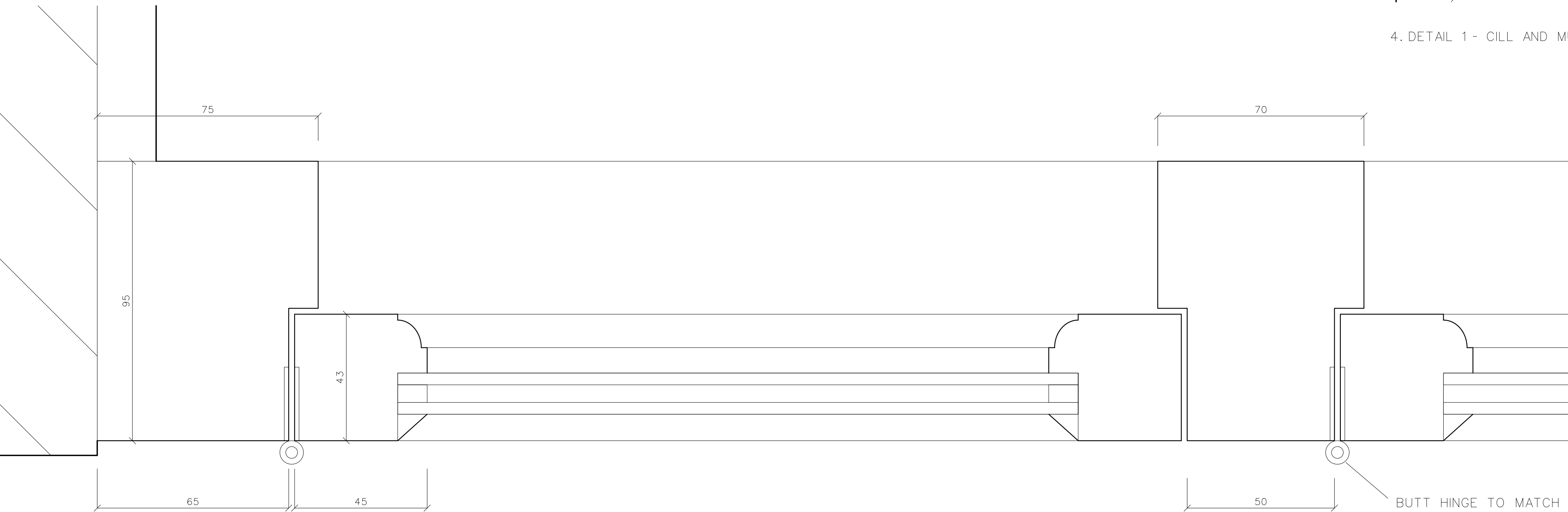
5. DETAIL 2 - FRAME AND CASEMENT. Scale 1:1
