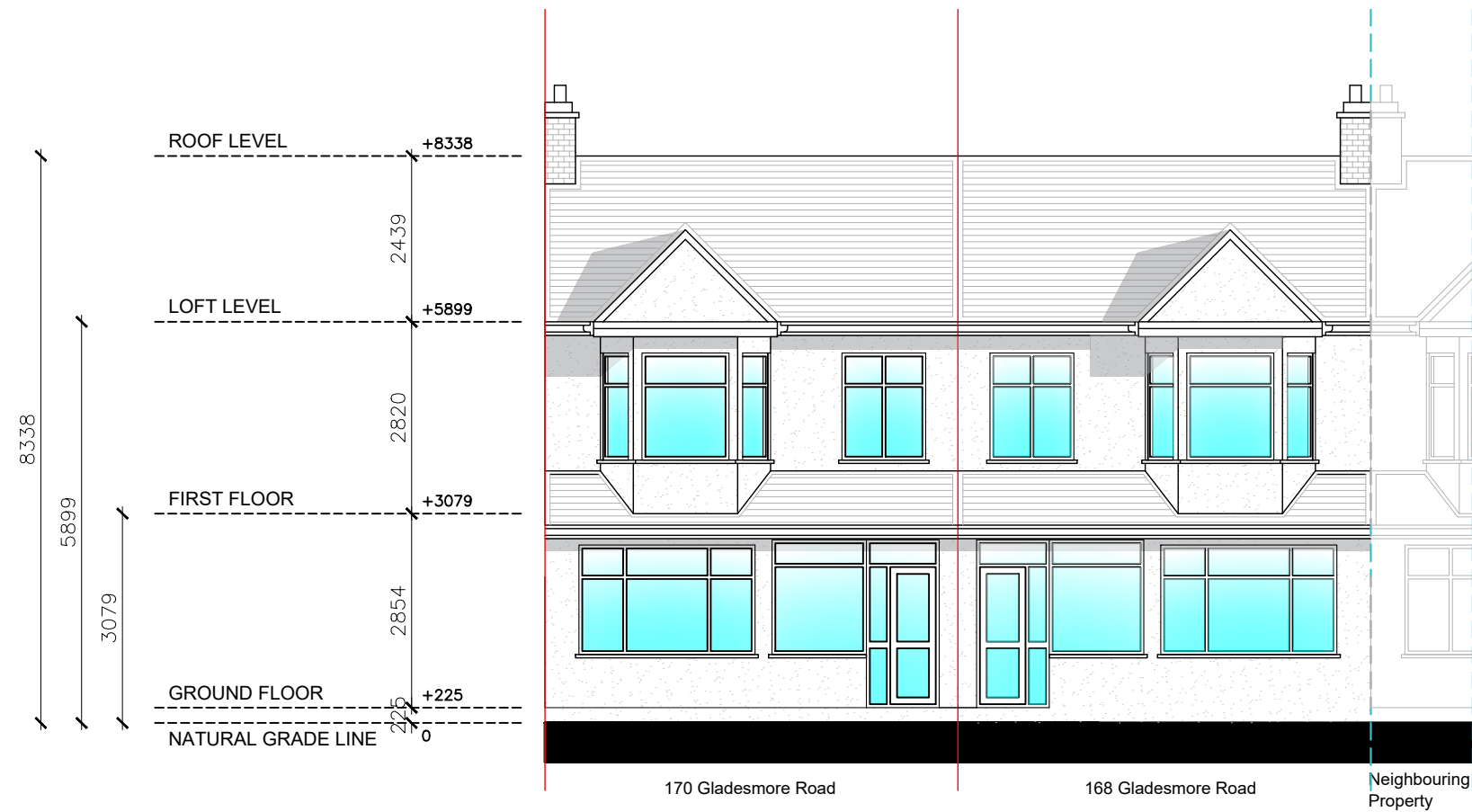
MAIN BUILDING NORTH-EAST ELEVATION (FRONT VIEW)
