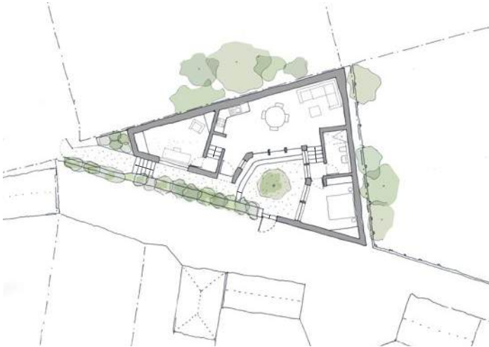
Pre-Application Update 80 sqm Pre-app Update: The second iteration of the design proposed a single storey structure which stepped down in level following the site topography. Level changes provided points of access from different points on the site, and also reduced the visual impact of the development
