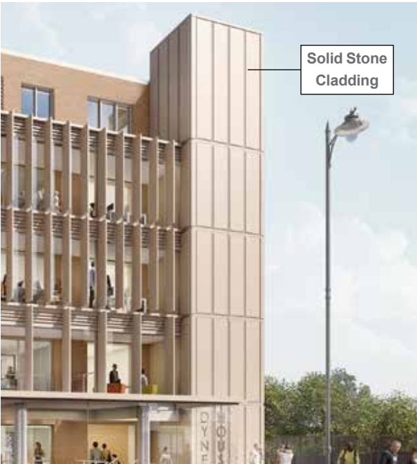
Stone Cladding on Lift Shaft
