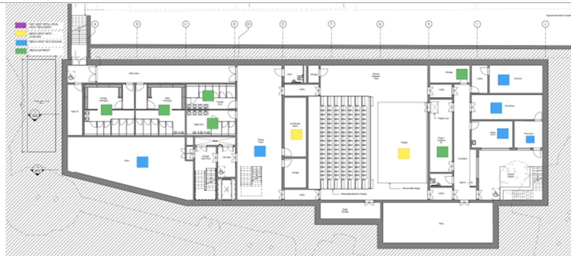
Figure 8: Basement Ventilation Strategy
