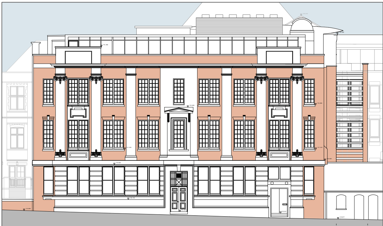
East elevation with rooftop plant area & observatory behind east block, north extension on right side
